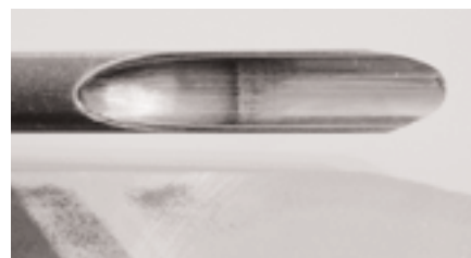
Milling marks in the flute of a gouge, above, and pits or milling marks on scrapers impact edge quality.
